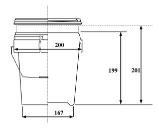
Measurements in millimetres
